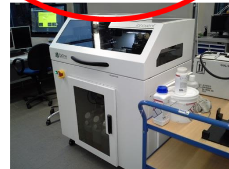
■ 3D Metal Printing - Binder Jetting approach (3DP) [HB]
