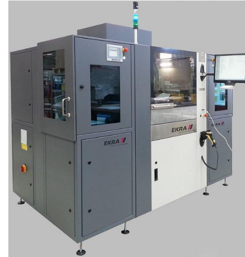
■ 3D Screen Printing (3DMP) [DD]
